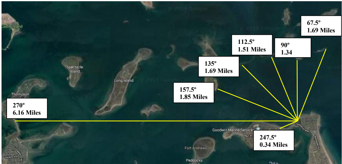
Figure E-2 Nantasket Seawall Shoreline Fetches
